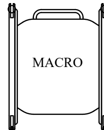
ROMAC MACRO HP 501 DUCTILE IRON WITH EPOXY COATING SOLID SLEEVE. (DISINFECT BEFORE INSTALL)
